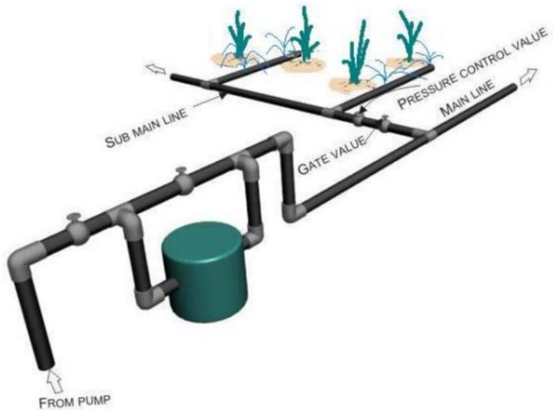
The sprinkler irrigation system
