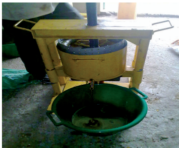
Figure 5 Pressing neem seeds using a manual press
