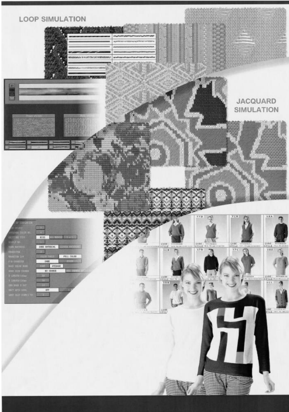
Fig. 12.3 The simulated knit package is mapped onto an image of a model to simulate the appearance of the final product. This image can also be used for evaluation and sales promotion purposes
