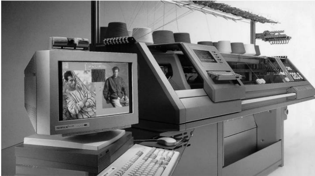
Fig. 12.2 Knitting patterns and programmes are quickly generated using automatic routines. These are checked and can be transmitted on-line to the CMS knitting machine. Simultaneous monitoring of production can also be achieved
