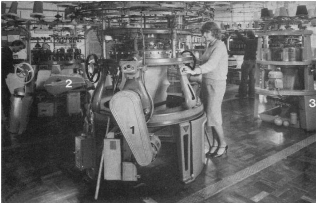
Fig. 8.3 Mechanically controlled circular knitting machines. 1 = plain cylinder and dial fabric machine; 2 = rib jacquard machine; 3 = double cylinder purl garment length machine.
