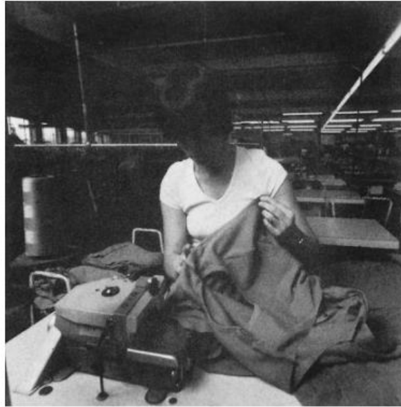
Fig. 6.3 Overlock seaming [Corah].
