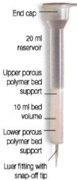
Fig 2. This is a depiction of a column used in affinity chromatography. The image comes from the Bio-Rad homepage.
