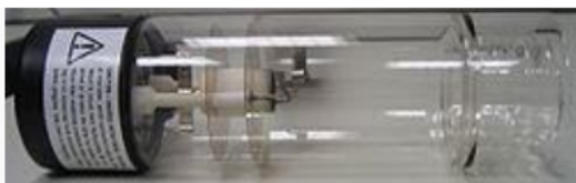
Hollow cathode lamp (HCL)
