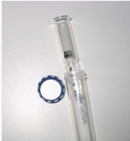
Figure: 11 A selectively permeable membrane can be mounted in a centrifuge tube. The buffer is forced through the membrane by centrifugation, leaving the protein in the upper chamber.
