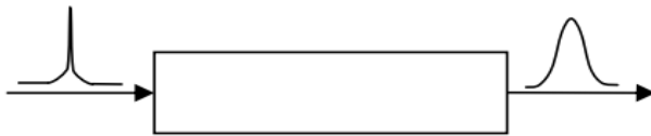
Figure 13. A pulse input can become an axially dispersed pulse output in a non-ideal PFR.
