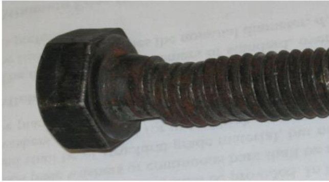
FAILURE OF BOLT IN DOUBLE SHEAR
