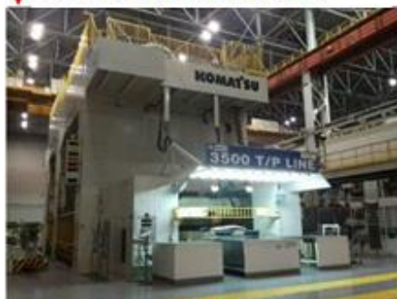
3500tonna Transfer liniya
