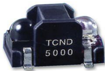
3.3-rasm. “Vishay Semiconductor” kompaniyasining TCND-5000 markirovkali sensori.
