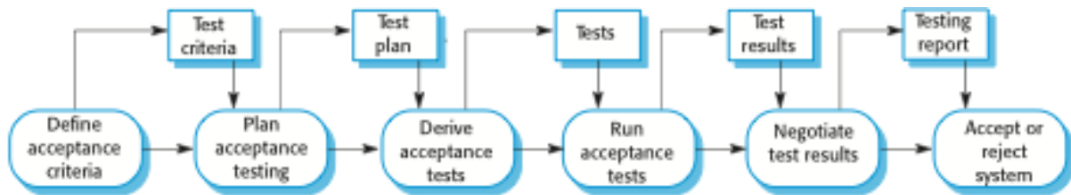
Figure 6. Acceptance Testing Process [1]
