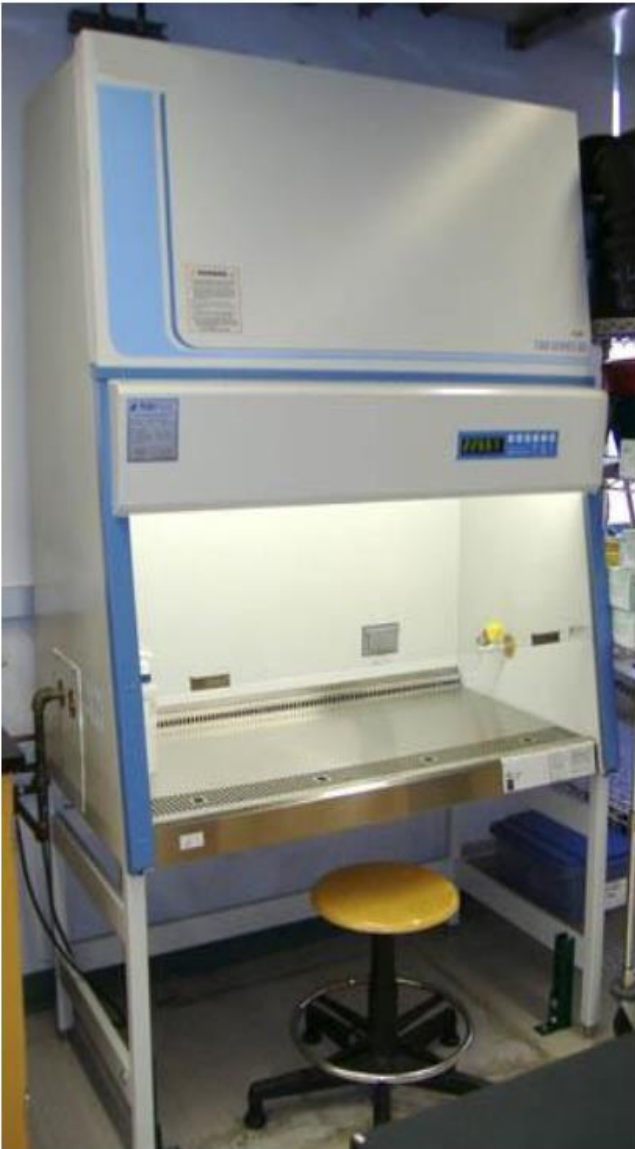
Figure 10. Laminar flow hood used to prevent contamination of solutions and cultures. Shown is a biosafety cabinet approved for work with BSL-2 organisms.
