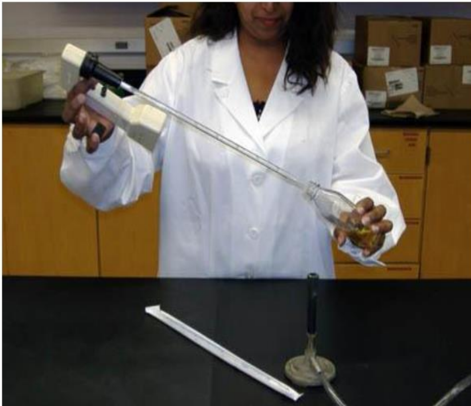
Figure 4. Aseptic technique. When aspirating liquids from a bottle, flask, or tube with caps, never place the cap on the bench. Instead, hold the cap in the same hand as pipette aid while manipulating the vessel containing the liquid with the opposite hand as shown.
