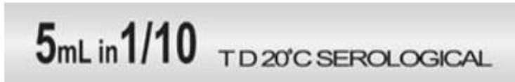
Figure 3. Serological pipettes are of two types: TC ("to contain") or TD ("to deliver"). Shown is the explanatory label of a TD 5 ml pipette.
