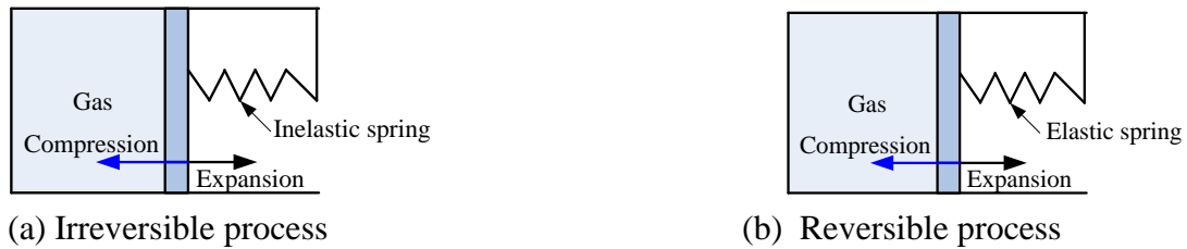
Figure 5.4. Process involving nonlinear or inelastic spring and process involving linear and elastic spring [2]
