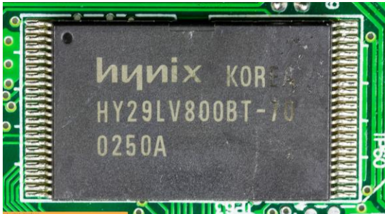
Spekking, Raimond. English: SEG DVD 430 - Hynix HY29LV800BT-70 - 8 Mbit (1M x 8/512K x 16) Low Voltage Flash Memory. November 3, 2016. Own work. https://commons.wikimedia.org/wiki/File:SEG DVD 430 - Hynix HY29LV800BT-70-4279.jpg .
