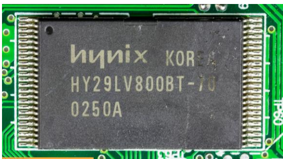
Spekking, Raimond. English: SEG DVD 430 - Hynix HY29LV800BT-70 - 8 Mbit (1M x 8/512K x 16) Low Voltage Flash Memory. November 3, 2016. Own work. https://commons.wikimedia.org/wiki/File:SEG DVD 430 - Hynix HY29LV800BT-70-4279.jpg .
