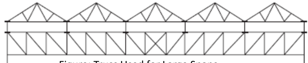
Figure: Truss Used for Large Spans
