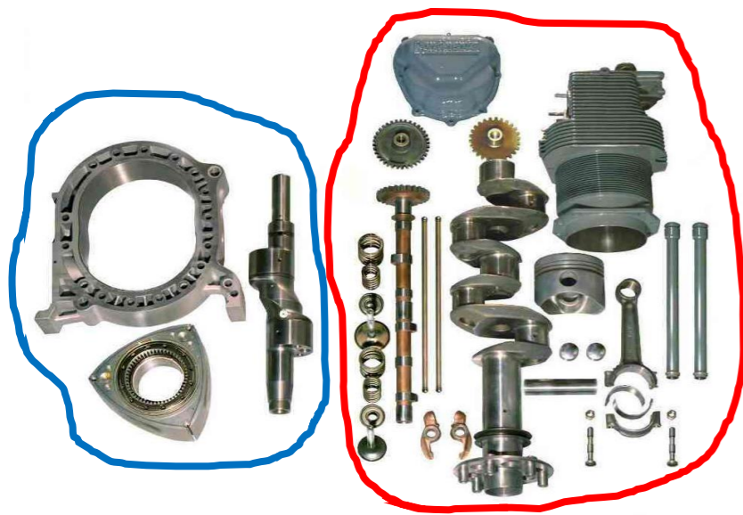
Rotary versus the aircraft piston engine.
