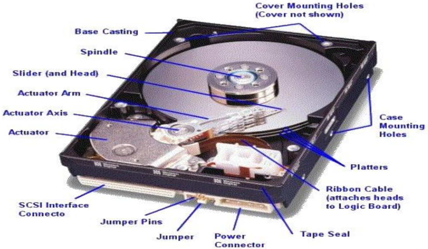
Figure 2: Components of a Disk Drive[2]
