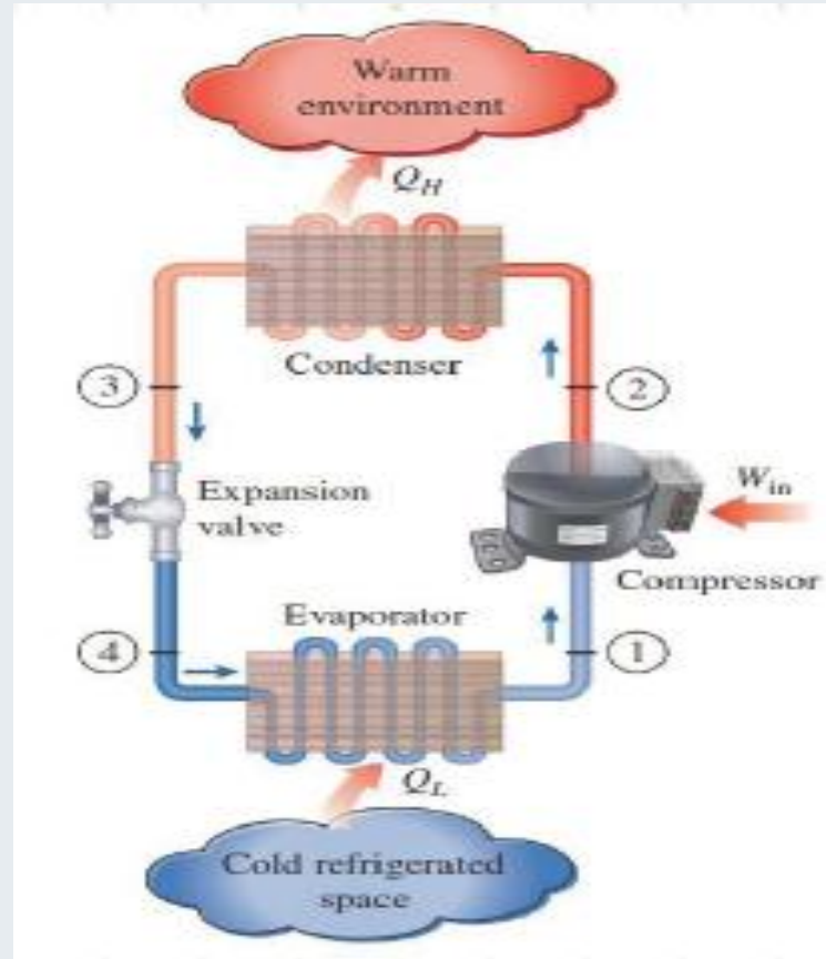
Figure 1: Components of a Refrigerator
