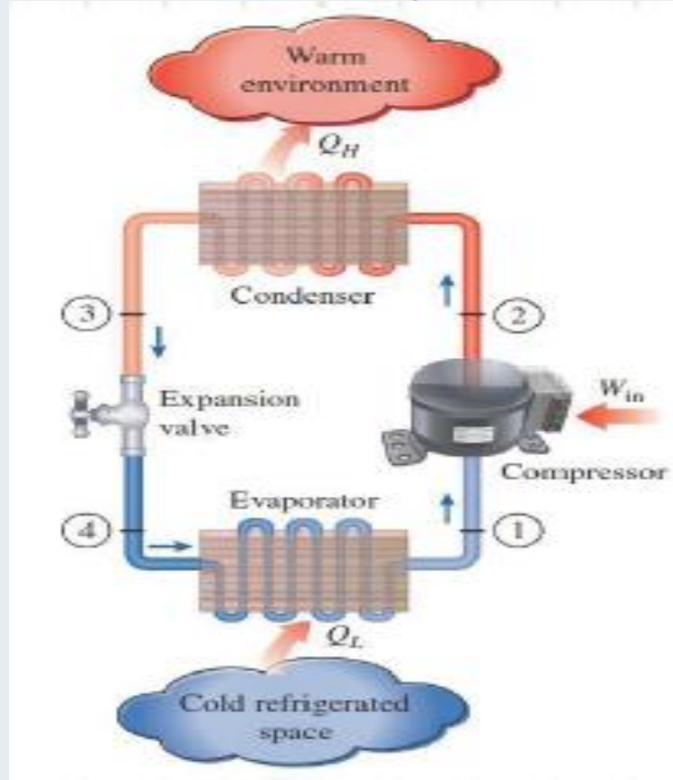
Figure 2: Components of a Refrigerator
