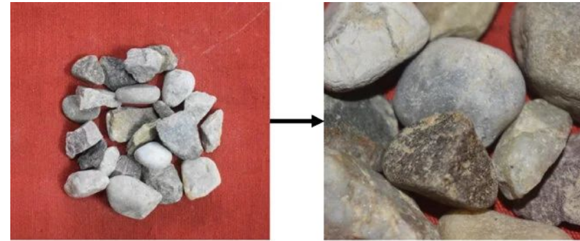
Rounded/irregular shape and smooth surface texture of the NCA
