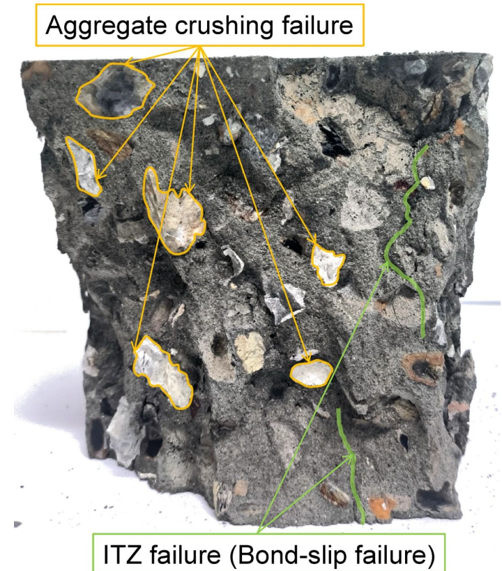
Failure modes during uniaxial compression tests. Adapted from Zhou et al.(2025)
