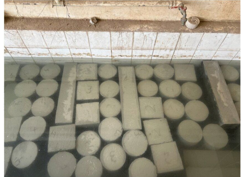
Concrete specimens submerged in water for curing Source: ResearchGate. (n.d.)
