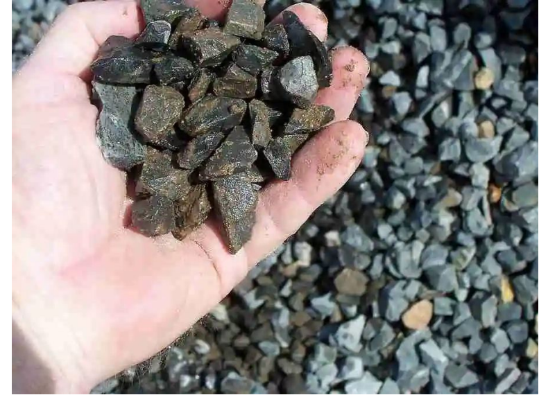
Moist aggregate Source: Suryakanta. (2015)
