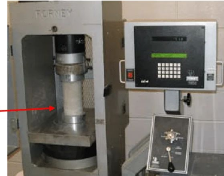
Compression test configuration (concrete cylinder). Source: ASTM International
