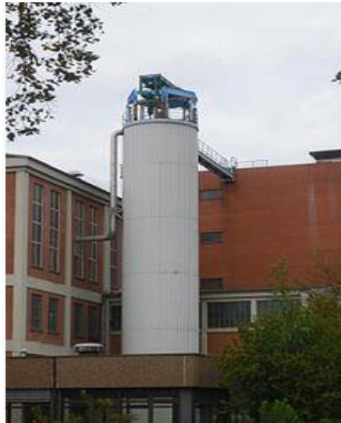
Vertical cooling crystallizer in a beet sugar factory
