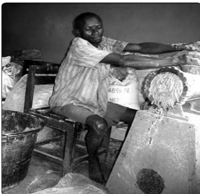
Figure 4.3-3. A simple pelleting machine is used to prepare fish feeds on the farm at Sagana Aquaculture Centre.
